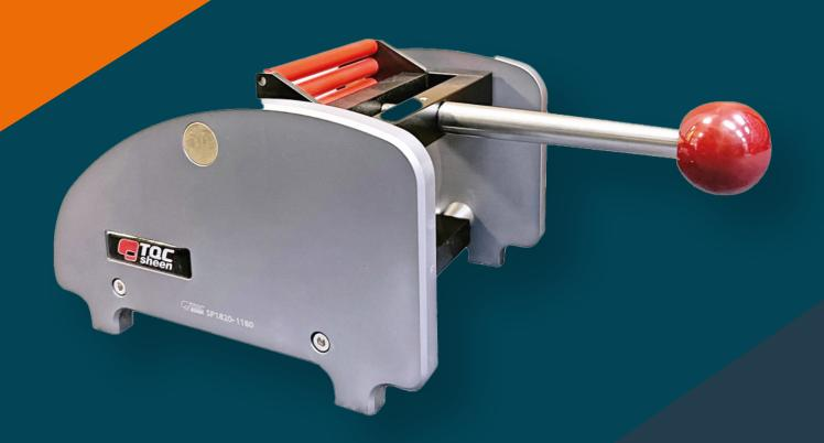
TQC Sheen Cylindrical Bend Test 100mm including Mandrel Set
