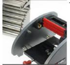
Sufficiently open the apparatus to insert the mandrel with the correct dia. turning the handle of the pressure rollers anti clockwise.
