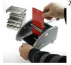
Place and secure a test-panel in the apparatus, positioned against the mandrel. Fix it upright into the clamp. The coated side of the panel should face outwards once the bend has been made.
