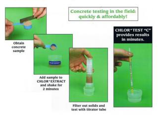
Cross contamination, from test to test, is eliminated through one time use of individual components. The components are pre-measured to ensure accurate results in parts per million. In addition no temperature correction is needed from 41F to 176F.
