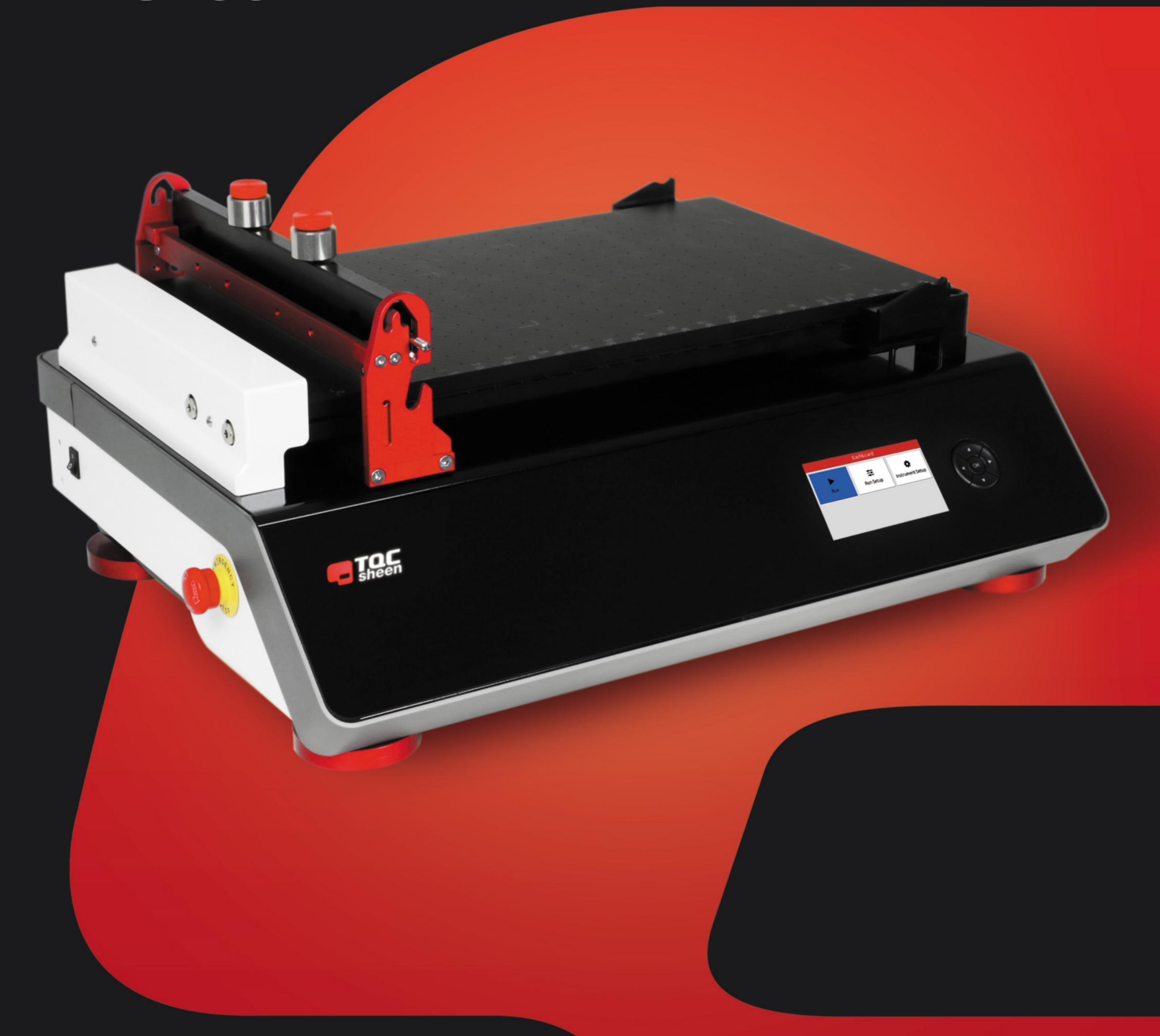
The AFA Standard provides a reliable basis to apply coating films to test charts, panels or foils in a uniform and reproducible way in order to eliminate variations caused by human factors. Variations in speed, pressure and direction of draw down cause irregularities. Other factors that may influence the result are the shear rate and the weight of the applicator.
