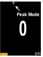
1.5.1 To zero the ATC, press the PosiTector menu button and select the "Zero" function.
