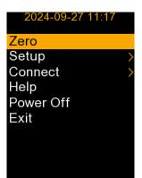
1.5.2 To toggle the Peak Mode, press the PosiTector menu button then select "Setup" and select / de-select Peak Mode.
